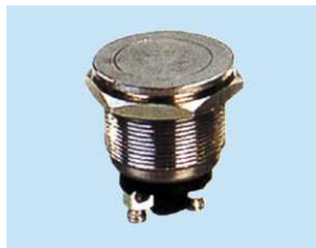
PS28B-2 OFF-(ON) 4 A 125 VAC; 2 A 250 VAC
