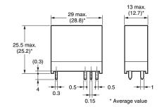
**Relays with PCB Terminals** (DPST-NO (2a) Relays)
