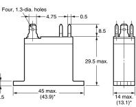
Mounting Holes (BOTTOM VIEW) Tolerance: ±0.1 mm
